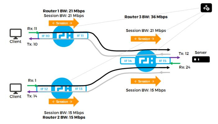
As shown above, the 128T Conductor collects bandwidth information from all the routers in a project and performs several calculations. The *Project-Wide Time-Averaged Bandwidth* is calculated for each 5 minute
