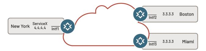
This deployment scenario is common when branches belonging to the same enterprise or different enterprises access the same service located at a common data center. Assume a service X is hosted in a data center located in New York. There are two branches located in Boston and Miami with overlapping IP addresses belonging to two different enterprises that need to access this service.
