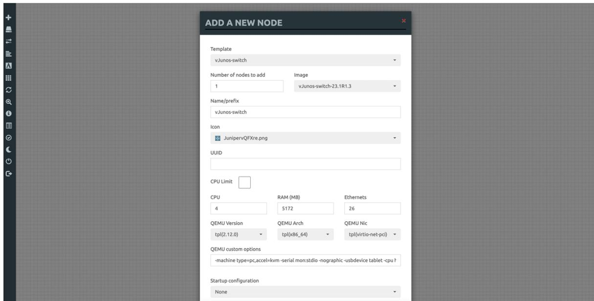
These devices can now be deployed and interconnected. To interconnect two devices, simply click on the orange icon seen when you hover over a node, as seen below:
