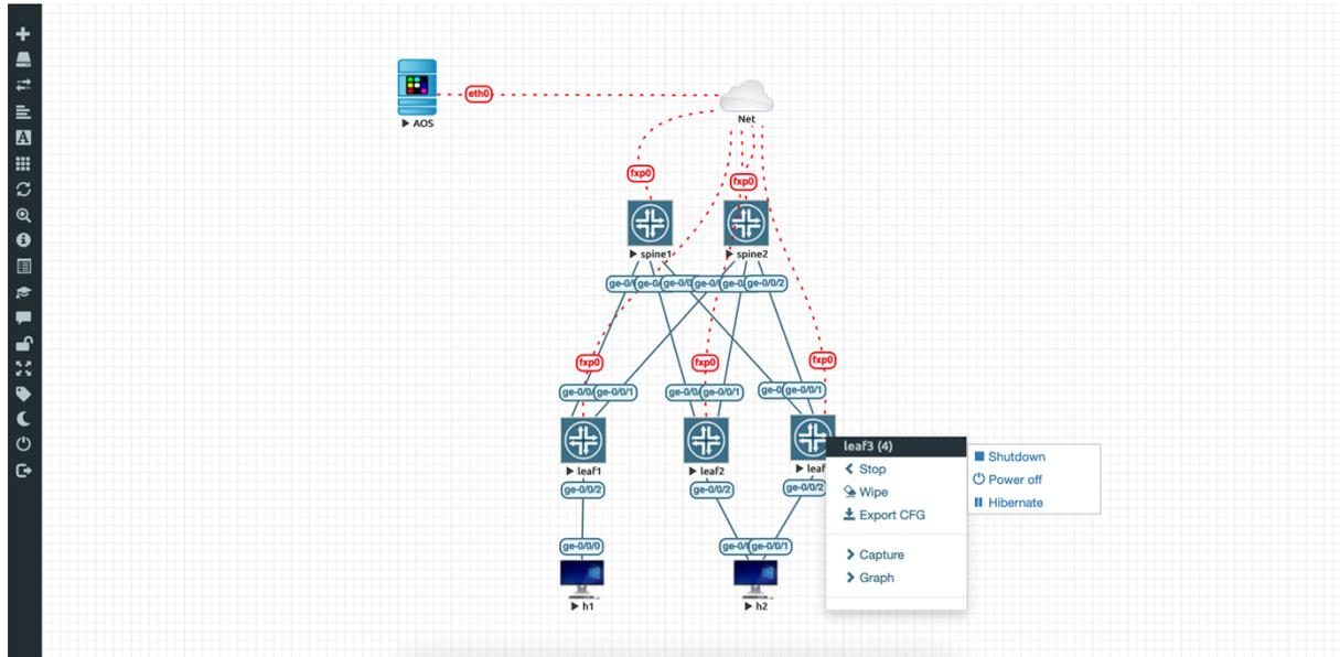
It is important to shut down the device gracefully (using the 'Shutdown' option). A power off (which is not graceful) has the potential of corruption the disk, rendering the device unusable. In EVE-NG community edition, issue a *'request system poweroff'* prior to shutting down the node via the UI, since these options are not available in the UI itself in this edition.
