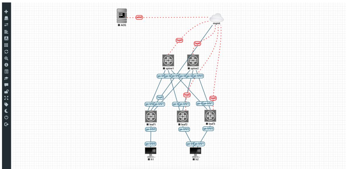
This topology is a typical 3-stage Clos fabric with two spines and three leaves. Two leaves (leaf2 and leaf3) are ES1 peers and connect down to the same host, h2.
