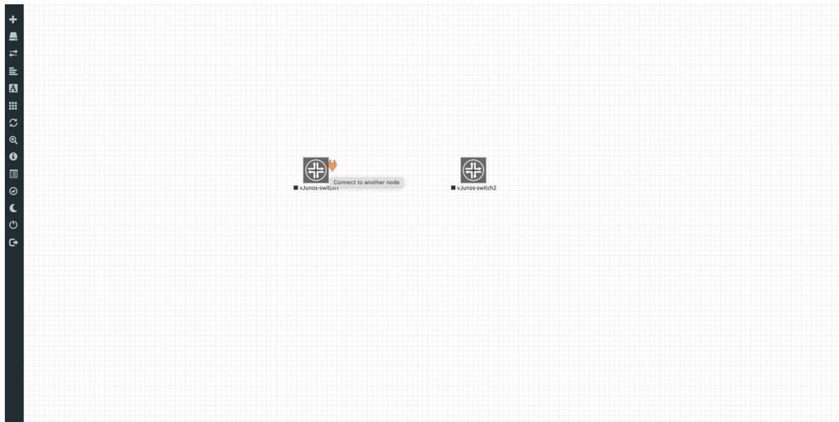
Once clicked, you can drag it to the destination node and let the connector go, which then gives you a pop-up to choose which interface is being connected on each side, like below:
