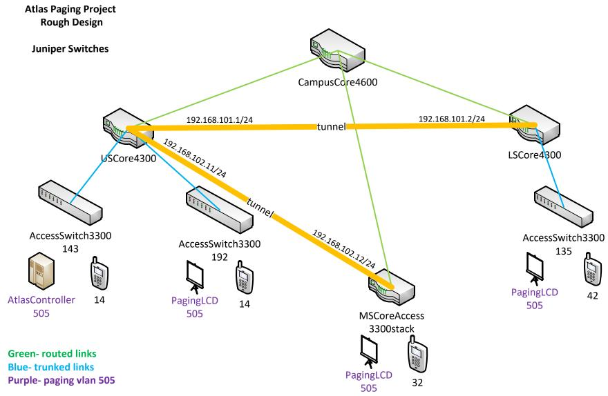
My proposal is create a separate vlan (505) for the lcd screens and the controller...and attempt to bridge that across the routed links. The other components stay put in their respective "voice vlans" as indicated by the phones...since they are routable and can utilize multicast.
