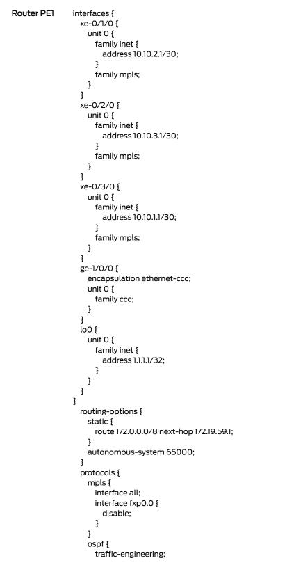
The relevant sample configuration for the spoke Router PE1 follows.
