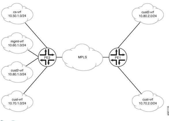
Figure 1: Layer 3 VPN Example for Demonstrating the Auto Export Feature
