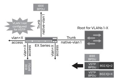
Figure 11: BPDUs received on the native-vlan will be treated as regular multicast packet.
