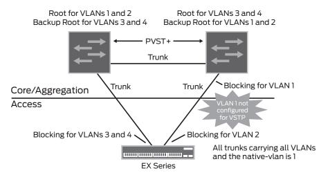
Figure 12: The upper-left switch is blocking the redundant link for VLAN 1.
