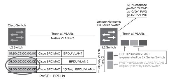
Figure 8: CST is still based on VLAN 1, even though the native VLAN is 2
