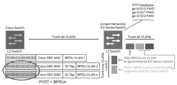
Figure 5: When EX Series switches receive BPDUs from a Cisco switch, only the IEEE STP BPDU is processed; the PVST+ BPDUs are flooded as regular unknown L2 multicast packets
