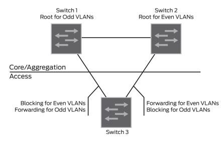
Figure 10: VLAN load-balancing between PVST+ (core/aggregation switches) and VSTP (access switch)
