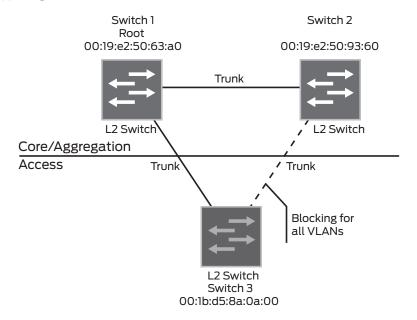
Figure 7: Juniper Networks EX Series Ethernet Switches at the core/aggregation layers running RSTP and Cisco at the access layer running PVST+; only one uplink on the Cisco switch is forwarding traffic
