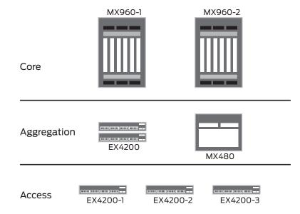
Figure 3: Typical three-tier enterprise switched network
