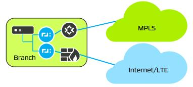
Certain sites require a dual router WAN design including regional offices and campus locations with large number of users. The dual router dual transport WAN edge design ensures complete link and router redundancy removing all single points of failure. Similar to single router dual transport WAN edge deployments the WAN links can be used in various degrees of preference. The diagram shows in-line topology however the design can ac-
