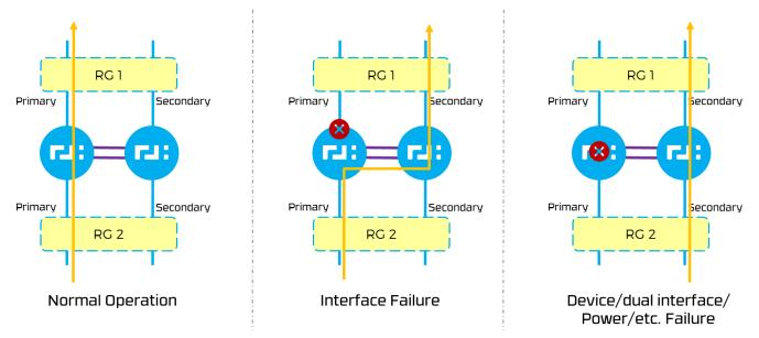
In case of a single primary interface failure, traffic will be routed through the fabric link to the secondary interface on the other router. This fabric link does not have to be a dedicated directly connected link. In case of process, device, component, or dual interface failures that completely disables the router passing traffic then the traffic switches over completely to the other router.
