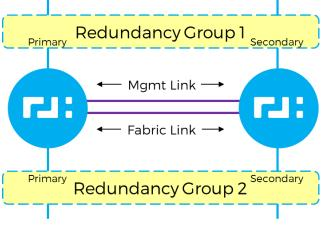
A fabric link between the routers is used to route traffic between them in case of failure. In the diagram these are shown as directly connected links but they do not have to be. Also the diagram shows two routers in a cluster for ease of understanding however there can be multiple routers in the cluster.
