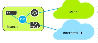
Most sites are expected to have dual WAN transports. These sites can be realized using a single router. This type of deployment supports link resiliency. It also ensures that a low-cost Internet path is used as the primary WAN interface. MPLS can serve as the secondary WAN interface. It can also serve as the primary WAN interface for high value traffic. LTE can serve as the path of last resort. The diagram shows inline topology however the design can accom-
