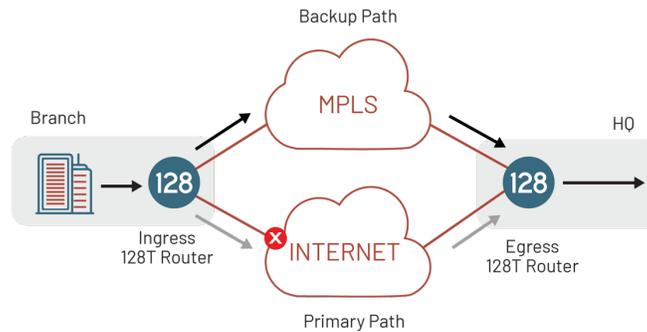
The traffic always flows over the Internet connection. In case of performance degradation, the sessions are moved to the MPLS connection. When the Internet connection is restored to acceptable performance, the sessions are moved back to the Internet connection.
