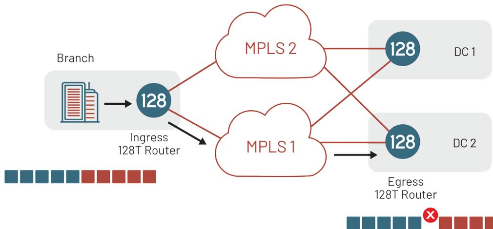
One method for flow performance monitoring is marking of packets in a specific session to different colors, thereby dividing the flow into different consecutive blocks. Packets in a block have same marking and consecutive blocks will have different markings. This enables the measuring node to count and calculate packet loss and/or delay based on each block of markers without any additional OAM packets.
