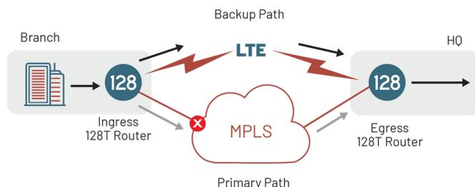
In case of failure the sessions are moved to the wireless connection. When the wired connection is restored the sessions are moved back to the wired connection.
