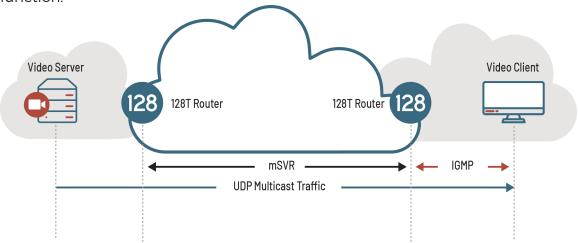
The 128T Session Smart Router implements IGMPv3. IGMPv3 is backward compatible so the 128T Session Smart Router is able to support clients running IGMPv1, IGMPv2, and IGMPv3. No changes will be required on clients when relying on 128T Session Smart Routers in the network for multicast.
